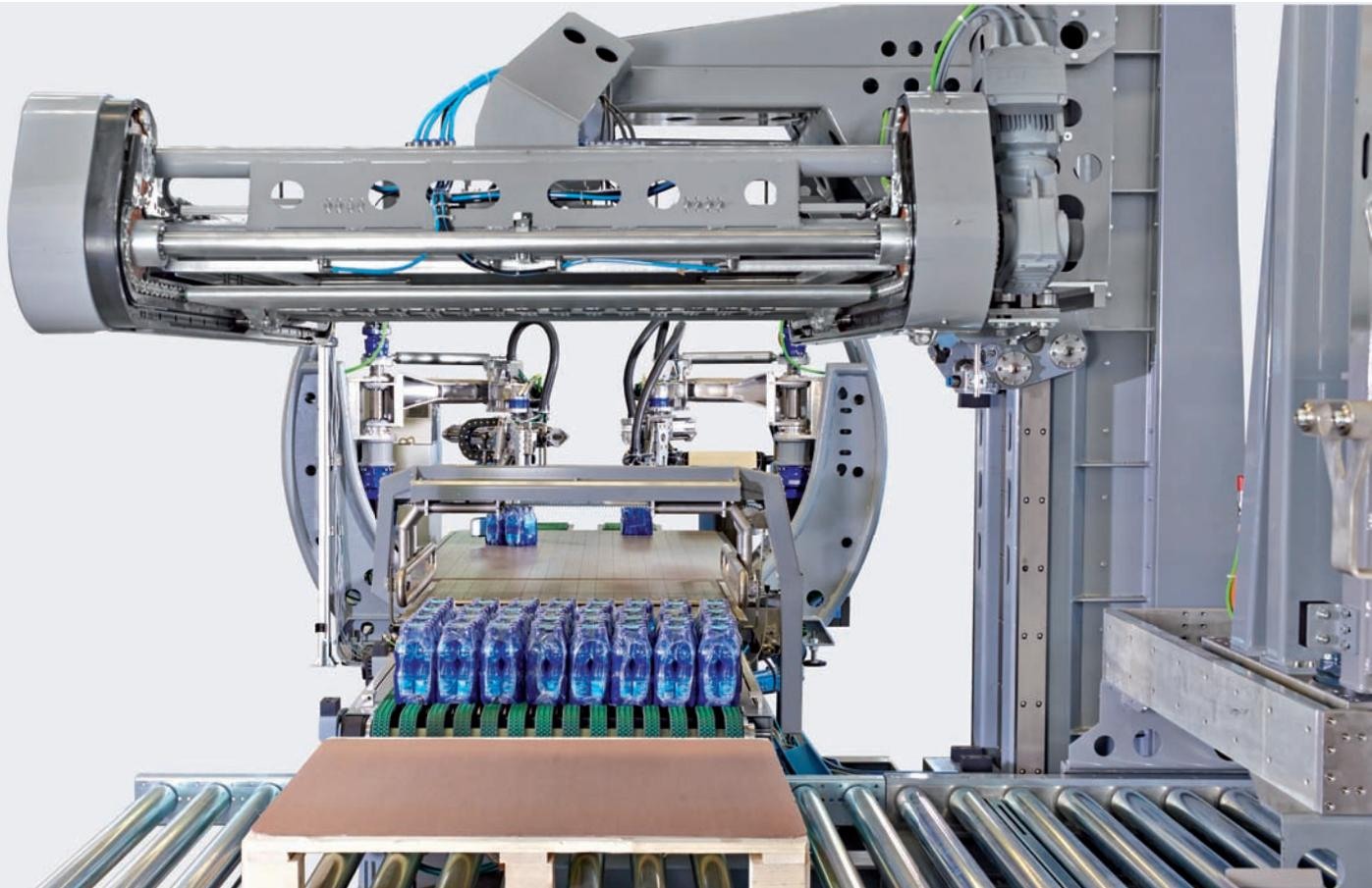
**GEA Procomac ARTIS EVO is the latest development in palletizing technology. ARTIS EVO uses a new (patent pending) system of layer handling to save space, reduce maintenance cost and maintain high speed production.**
