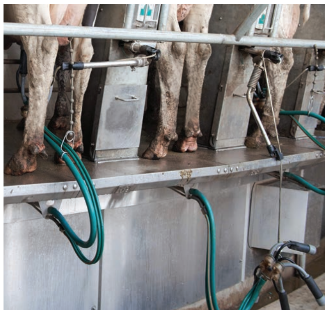
6. Unit Drop-down: The PosiForm swings the milking unit down and out of the way after milking, providing operators unobstructed access to the udder.
