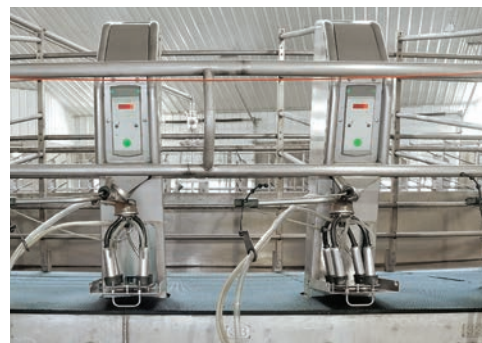
Integrated C.I.P. panel — folds down for use and quickly stows away for milking. Built with a stainless steel pillow and rubber jetter cups.
