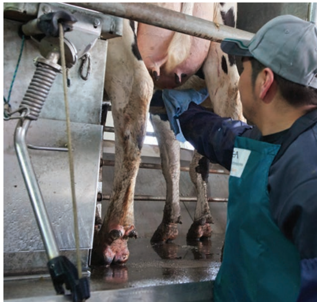
2. Cow Prep: The PosiForm arm keeps the milking unit safely out of the way of the cows and operators during prep procedures.
