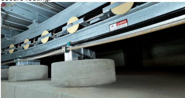
Heavy-duty platform — ruggedly designed roller carriage requires no lubrication and eliminates the need for bearings that wear out. It also runs quieter for a more pleasant parlor environment.
