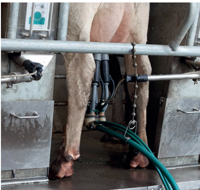
5. Unit Removal: After milking, the PosiForm arm removes the milking unit straight off the udder (not at an angle) and away from the cow's legs.
