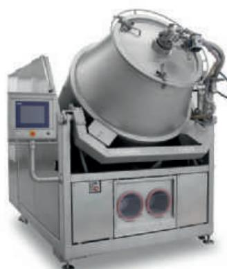
Both machines can also be applied for regular mixing or tumbling and massaging, and are not limited to defrosting. Please note that there are specific requirements for the steam system needed in vacuum defrosting.
