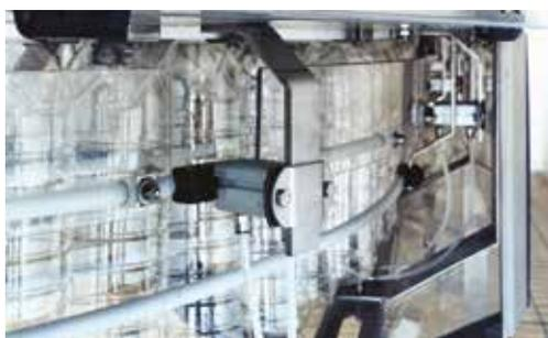
friction bottle guides design give Convair the capability to handle any kind of bottles including tapered neck bottles.
