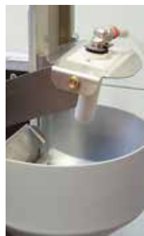
Pulsed compressed air cleaning
