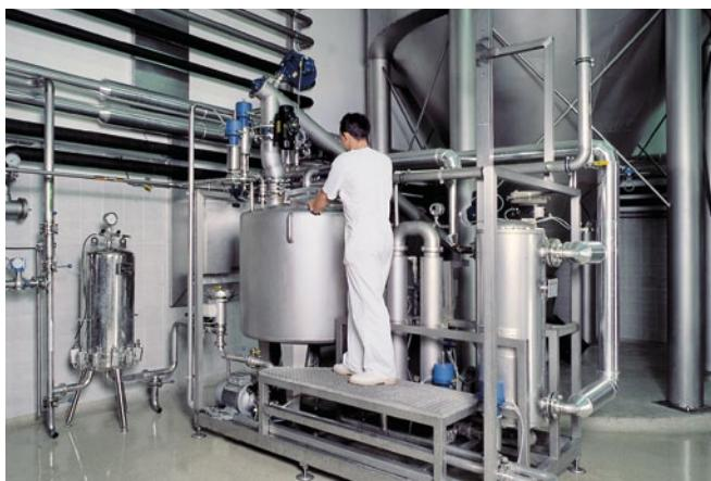
The finished syrup is now mixed with degassed water and beer to form a finished beverage. Flash pasteurization and carbonation of the finished beverage follow.
