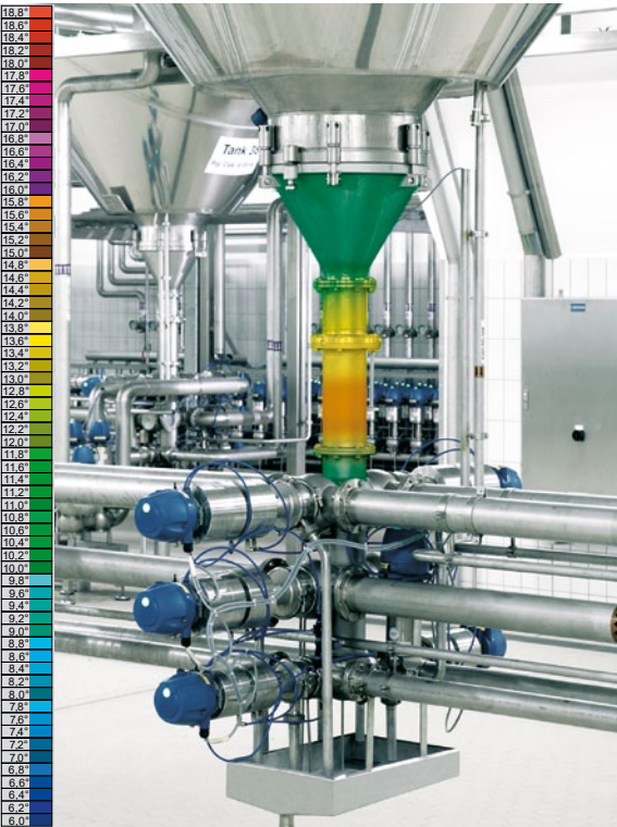
Temperature profile in the tank outlet and the ECO-MATRIX™ tank tree
