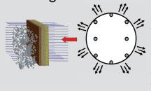
During normal filtration the filter bags are held in place by the wires of the bag cages, preventing collapsing by differential pressure. During bag cleaning phases, low pressure pulses of cleaning air are injected into the filter bags.
