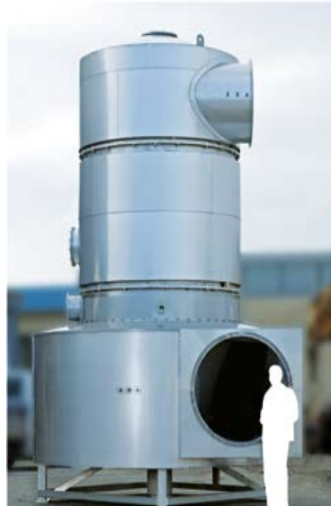
The SWIRL FLUIDIZER® is available in several sizes. This picture shows the drying chamber for a unit designed to dry more than 12 tons of powder per hour.
