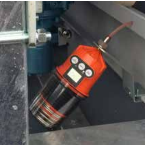
Auto greaser fitted to carriage roller assembly.
