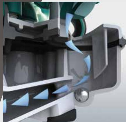
The automatic vacuum switching system only activates the full vacuum for each of the four quarters when the teat cup has been closed by the teat. The vacuum remains stable and this means that air slurps and slushing contamination of the milk path are virtually eliminated by our IQ system. The result: an easy way to guarantee clean milk.
