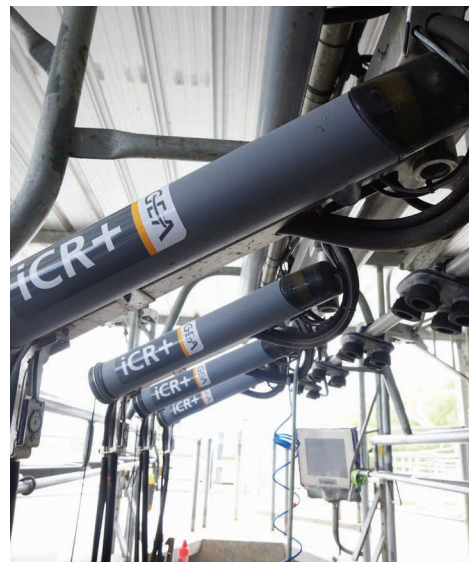
iCR+ intelligent cluster removers, iNTELARM+ swing-over arms and iASSIST swing down jettors standard with Easy Flow
