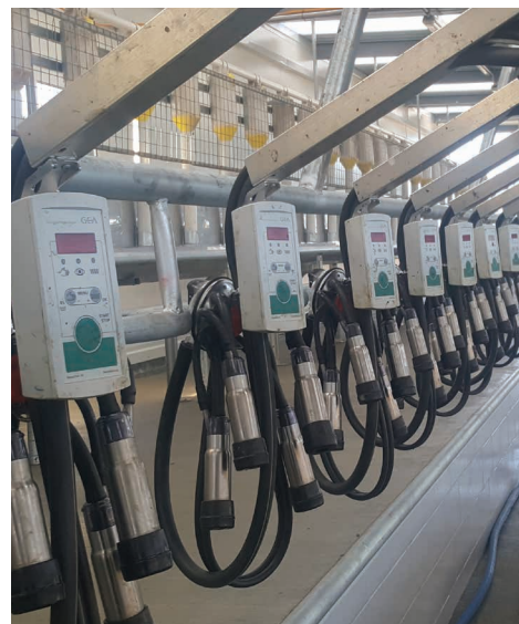
Add individual cow ID, milk metering with ICAR approved DemaTron 70 control panels
