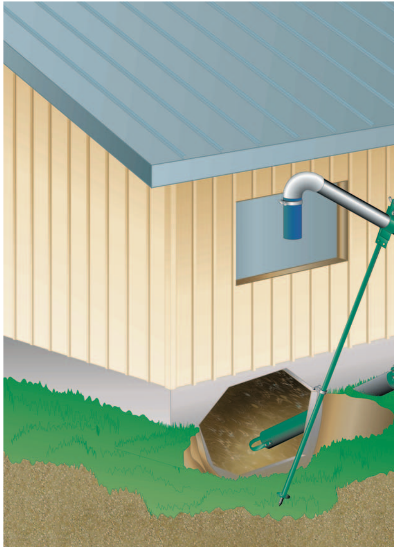
Hand primer pump with 6" (152 mm) gate valve
