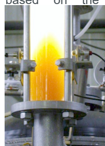
A W6 wash column illustrating the sharp separation between the washed ice crystals on the top and those still surrounded by concentrated product on the bottom.
