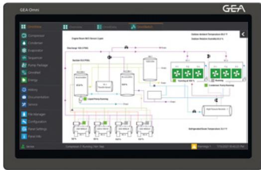
This OmniSketch example illustrates a typical refrigeration system layout with key status information.
