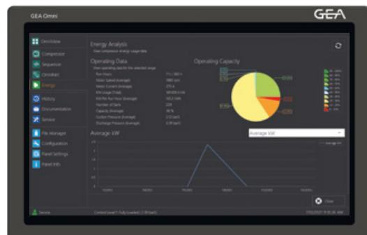
GEA Omni's Energy Management function allows operators to evaluate system energy usage and adjust to reduce operating costs.
