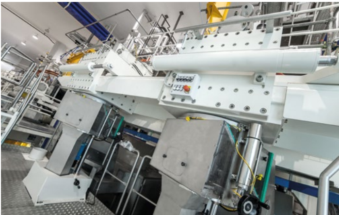
Pennaut 2T installed in a 6 t/h short-cut dry pasta line.
