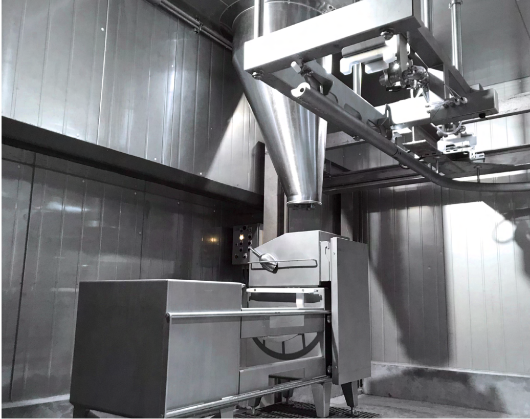
Tray filling station with buffer vessel and trolley elevator installed in a +5°C room.
