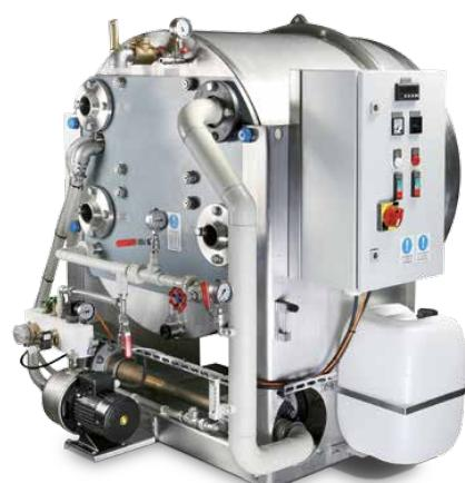
The SWD (GEA **SeaWaterDistiller**) works on the well-known vacuum distillation principle. Waste heat from the main engine on board is utilized as heating medium for evaporation. The evaporation takes place in the evaporation plate bundle located in the lower part of the housing.
