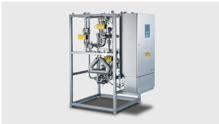
The GEA standomat has been designed for continuous cream fat or milk fat standardization in combination with the separation process.
