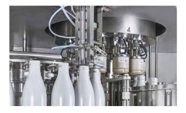
**Versatile solution for HDPE/PET bottles applications.**Foil infeed system and GEA patented induction sealing turret of GEA aseptic sterile solution.
