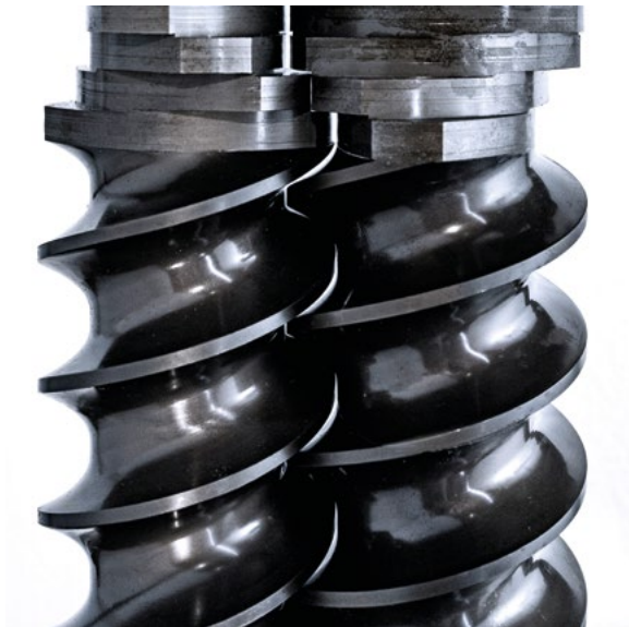
Two co-rotating screws composed of modular sectors.
