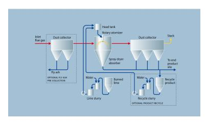
The Spray Drying Absorption process – a semi-dry flue gas desulphurization and cleaning process – facilitates a reaction efficiently transforming gaseous pollutants such as e.g. SO2, SO3, HCl, Hg, and dioxins into a slaked lime Ca(OH)2 absorbent to form a stable and dry powdery product that is easy to store and transport.
