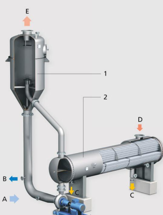
**A = Product, B = Concentrate, C = Condensate, D = Heating steam, E = vapor, 1 = Flash vessel/separator, 2 = Calandria**
