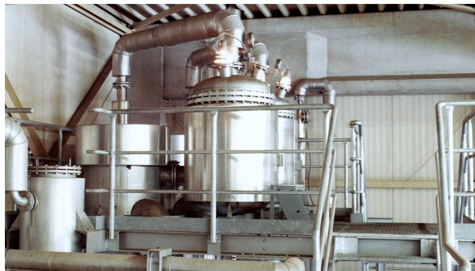
Where the boiling chamber of the circulation evaporator is divided into several separate chambers, each one equipped with its own liquid circulation system, the heating surface required for high final concentrations can be considerably reduced compared to an undivided system based on the same evaporation rate.
